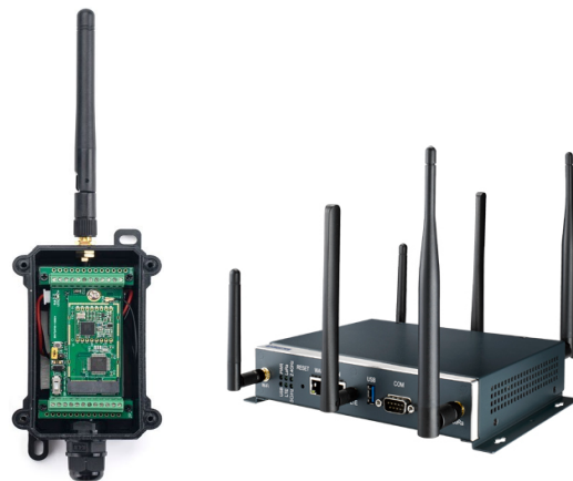
Fig. 1. Dipole antennas on a LoRa sensor node [16] and on a LoRa network gateway [17]
