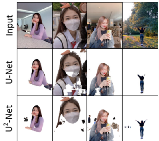
Fig. 4. Background-removed outputs from U-Net [15] and U2-Net [3]. Outputs from U2-Net show smoother and noiseless boundaries
